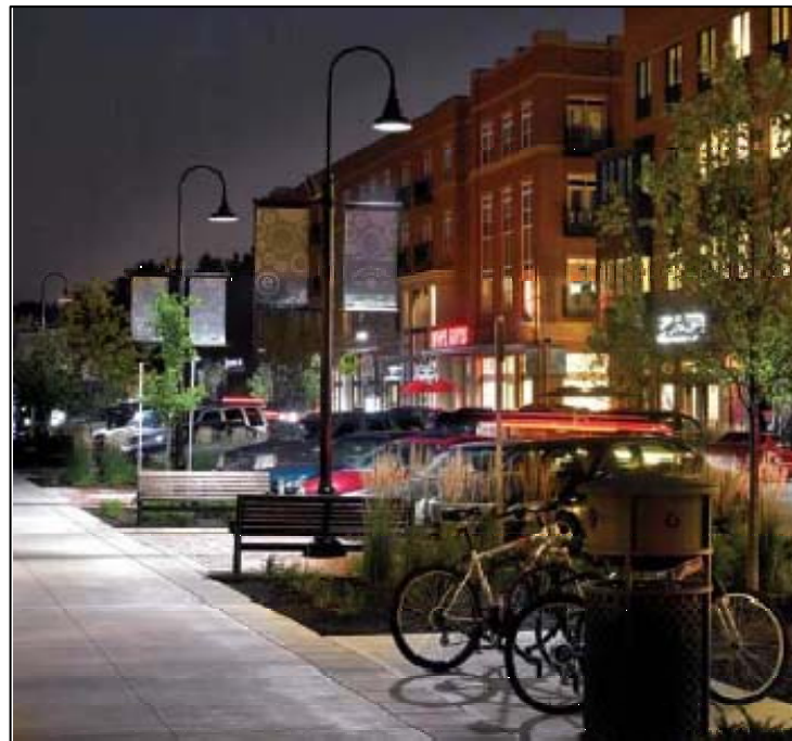
This photo shows pedestrian-scaled lighting in South Bend, Indiana. Overhead lighting on pedestrian-oriented streets should be low enough to the ground to illuminate walkways and the faces of pedestrians.
