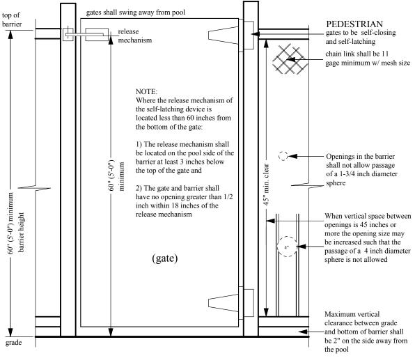
Any decorative design work on the side away from the swimming pool, such as protrusions, indentations or cutouts, which render the barrier "easily climbable" is prohibited.
