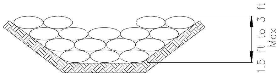
GRAVEL BAG CHECK DAM ELEVATION
