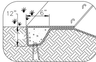
TERMINAL SLOPE AND CHANNEL ANCHOR TRENCH
